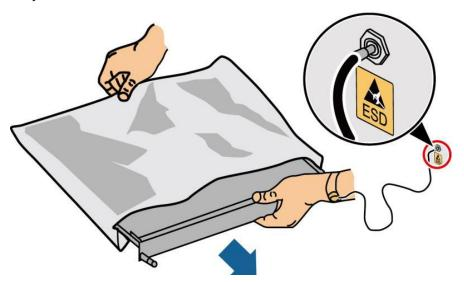
Fig. 1-1 Diagram of wearing ESD strap
